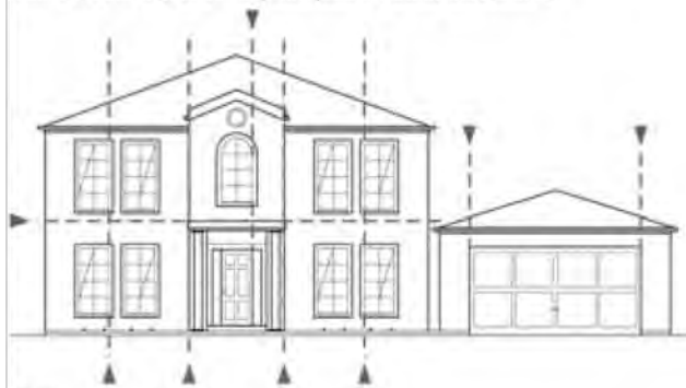
Unitex Base Board: Guide for Control / Expansion Joints - Front Elevation (use same principles for other elevations)
